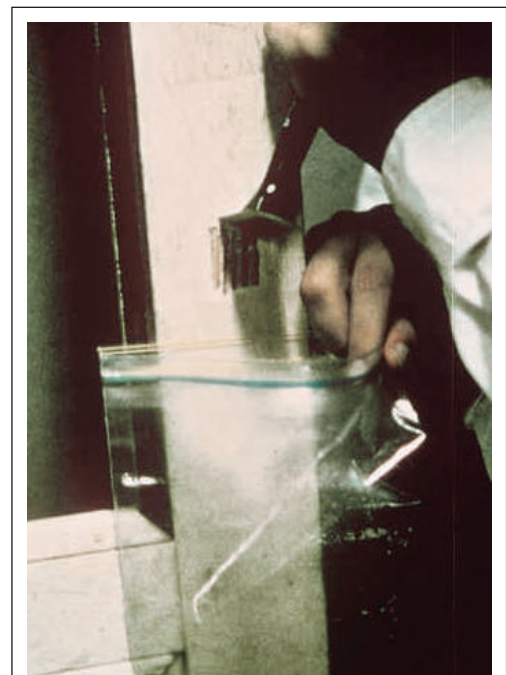
FIGURE 7.5 Removing paint-chip sample.
