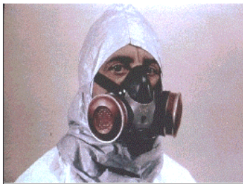
Half Face Air-Purifying Respirator Negative Pressure
