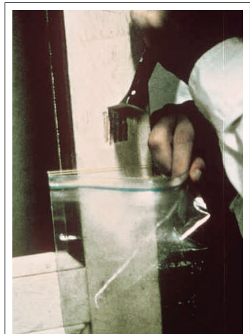
FIGURE 7.5 Removing paint-chip sample.
