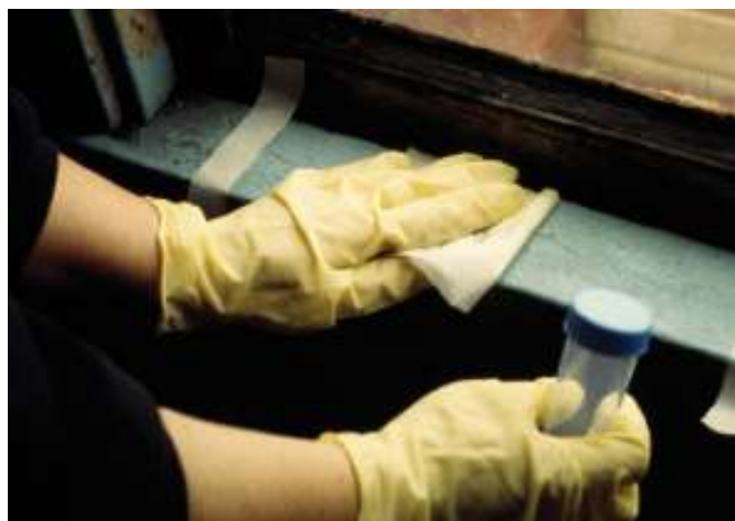
FIGURE 5.16 Dust testing a window sill to determine the presence of a friction hazard.
