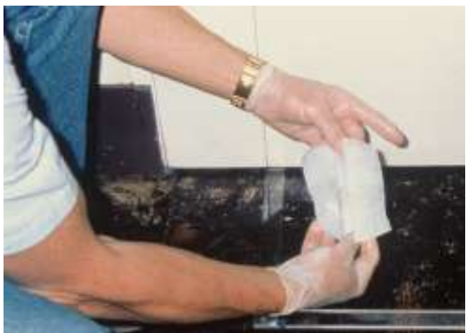
FIGURE 5.11d Folding wipe over for second pass.
