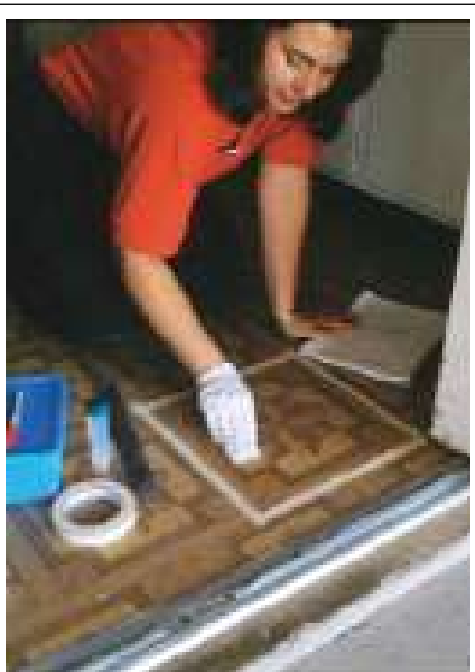
FIGURE 5.12 Floor sampling in high traffic area near entry.
