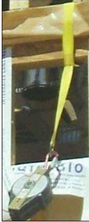
Figure 24 - A reusable strap anchoring a retractable lifeline.
